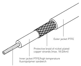
High temperature resistance heating conductor
