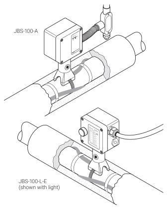
The nVent RAYCHEM JBS-100 kit is designed to connect power to a single nVent RAYCHEM BTV, QTVR, XTVR, HTV or VPL industrial parallel heating cable.
