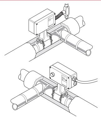
The nVent RAYCHEM JBM-100 kit is designed to connect power to up to three nVent RAYCHEM BTV, QTVR, XTVR, HTV, or VPL industrial parallel heating cables.
